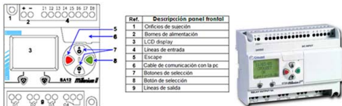
Figura 2.14 PLC Millenium II. Crouzet USA.com
