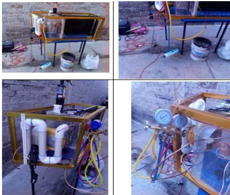
Figura 16 Compressor installation, system vacuum, charging and calibration of the refrigerant gas pressure
