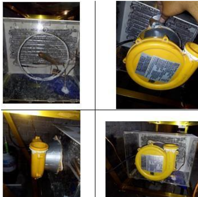
Figura 14Air recirculation blower
