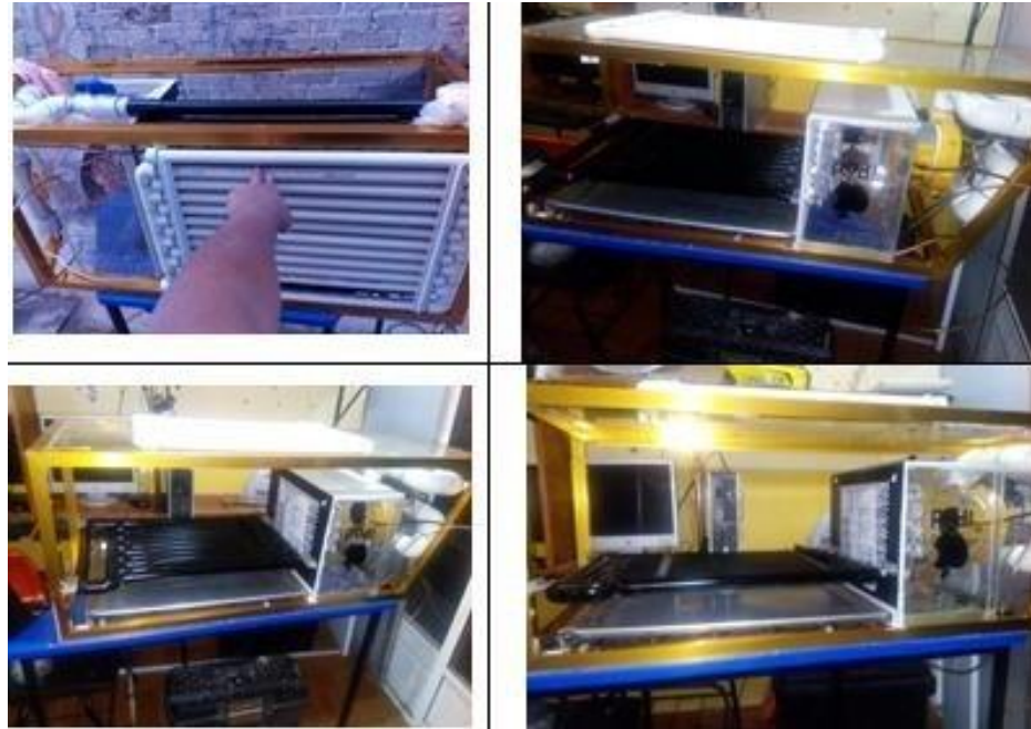
Figura 17 Heat pump and dehydration chamber assembly
