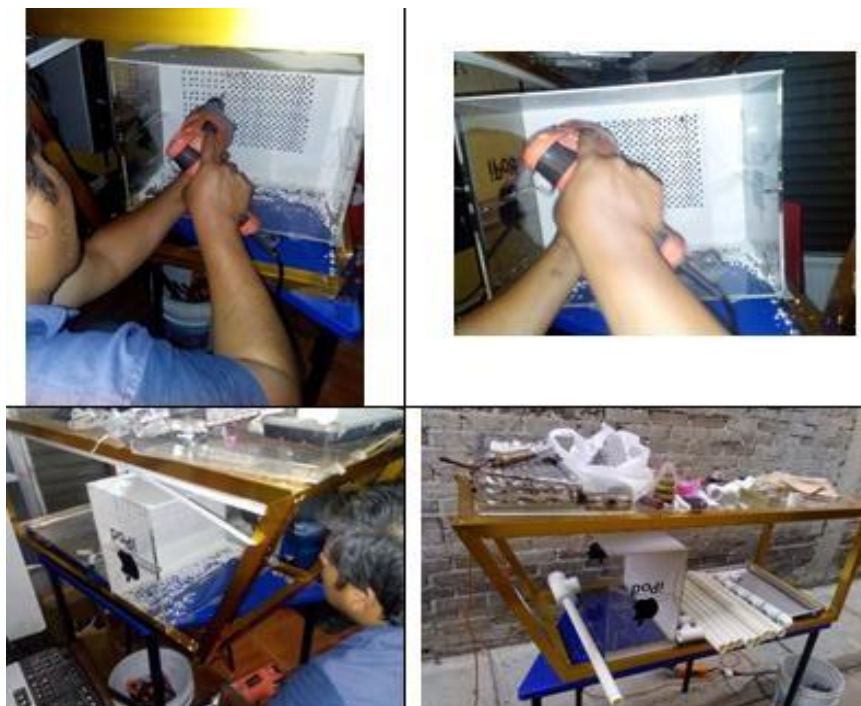
Figura 12 Initial phase of construction of the dehumidification chamber
