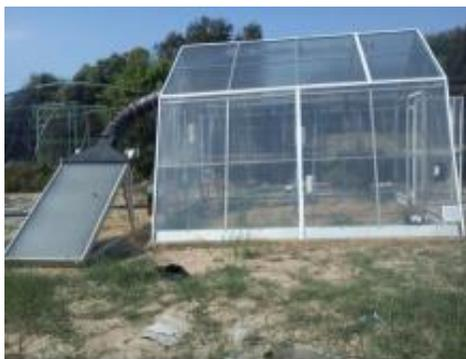
**Figure 2-3.** Greenhouse solar dryer used by Hamdi & Kooli (2018).
