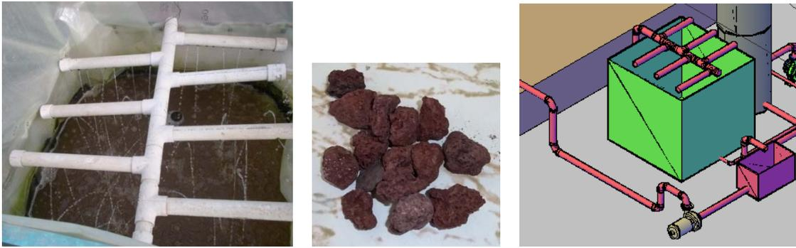
Fig. 3.14. First submerged biofilter and its water distributor mounted above the biofilter media, Tezontle used as a media for the submerged biofilter with mean diameter 1 cm.
