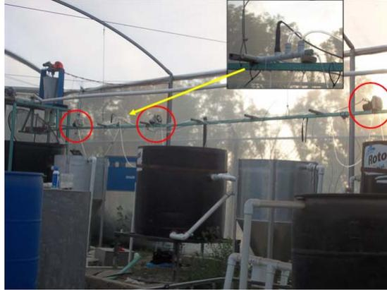
Fig. 3.30. Overview of the peristaltic pumps mounted over the tanks and the hydraulic head system.
