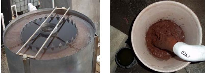
Fig. 3.10. The solids that captured in the channel of the separator and that discharged from the bottom.
