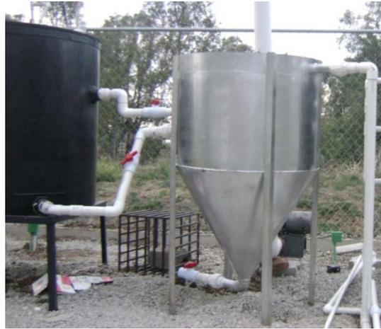
Fig. 3.5. Separator with two inlets one from the tank bottom to the separator center and the other from the upper part of the tank to the lateral side of the separator.
