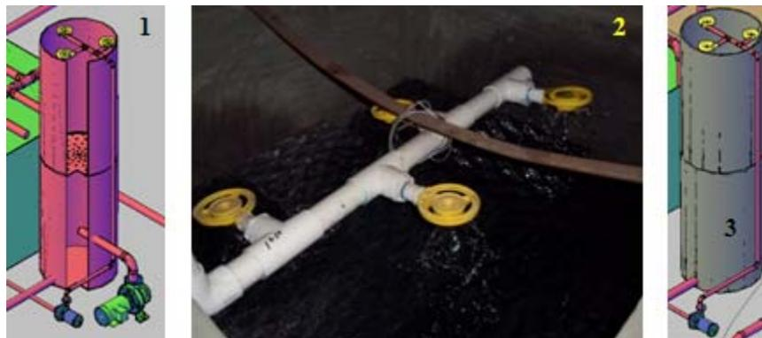
Fig. 3.23. The three different aeration techniques that were used (1) spray column aerator (i.e. water pump with air fan), (2) Gravity aerator, and (3) spray column aerator with water pump only.
