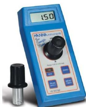
Fig. 7.3. Ammonia Photometer (Low Range) 0 to 3 mg/L **HI93700**
