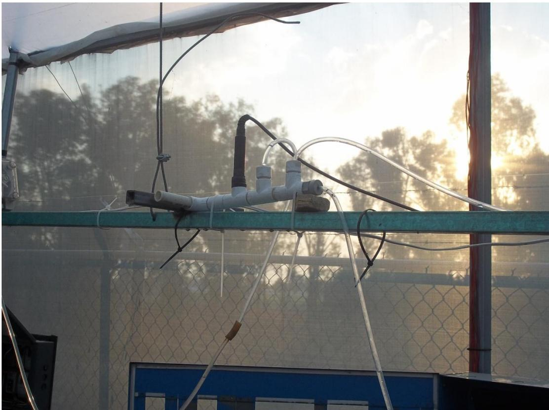
Fig. 8.13. Three inputs of the samples of three tank that was extracted by the peristaltic pumps.
