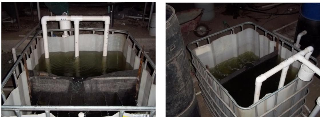
Fig. 3.15. The biofilter of Tank 3.
