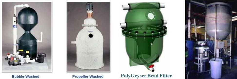
Fig. 2.11. Bead filters are distinguished by the way the beads are washed. The bubble washed unit is cleaned by draining and the propeller-washed units are intermittently cleaned by a propeller and The Poly Geyser Bead Filter is the next generation in Bead Filter technologies primarily through its automatic pneumatic backwash mechanism Microbead Biofilter.
